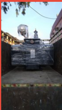
500kva HT Transformer Level-2
